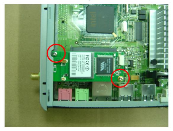
5. Connect the wireless cable (Module side) as below picture:
