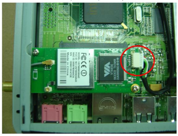
6. Connect the wireless cable (Board side) as below picture, please note the red line direction:
