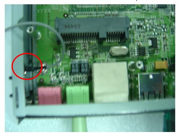
3. Screw the antenna connector as below picture:
