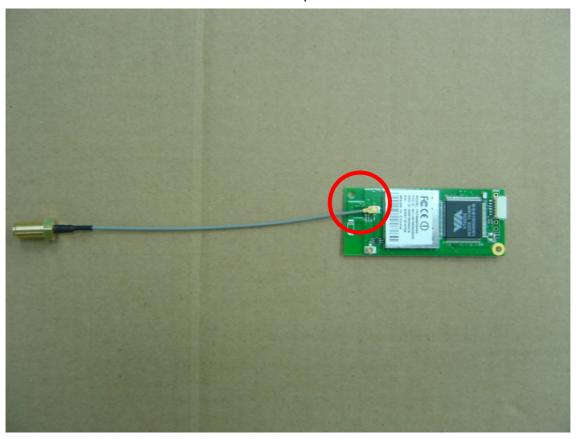
2. Make the antenna connector cross the chassis as below picture:
