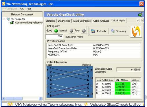
Cable Information will still function even the link is down, it will show the termination status and the distance of faulty point.
